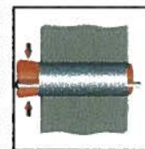
3b. Install plug around cables (optional: CP 618 Putty Stick forced into interstices of cables)
